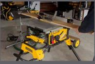
DeWalt's DWE7491 still tops the charts years after its initial launch. We love the rack-and-pinion fence system, there's plenty of power from its 15-amp motor, the accuracy is excellent, it has a wider table than many, and the rolling stand gives it a nice stable platform. www.dewalt.ca
