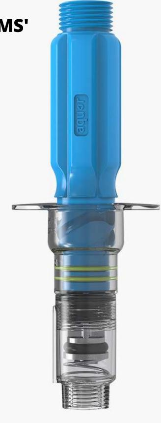
Conventional spigots have a flawed sealing mechanism. The friction of rotating compressing a rubber washer onto a brass valve seat causes wear, which creates leaks. Aquor's hydrant uses water pressure to keep its valve closed, rather than a screw- tightened assembly. This valve design seals with the same pressure and motion every time. Unlike a standard hose bib, the hydrant cannot be over-tightened.
