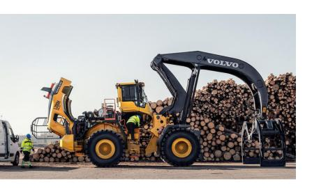
Volvo Construction Equipment launched the new L200H high lift wheel loader in North America. The industrial loader features a 27% increase in lifting capacity and a 13% larger grapple than the L180H model it replaces. This means the L200H can handle more timber per hour.
